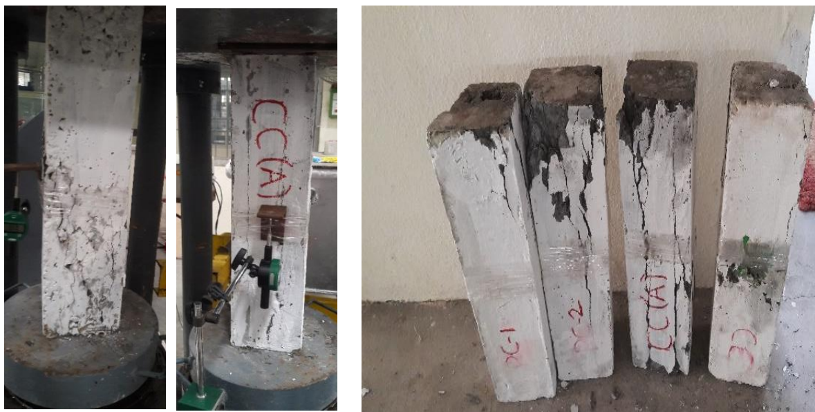
Fig 11. Typical failure mode of the column specimens
